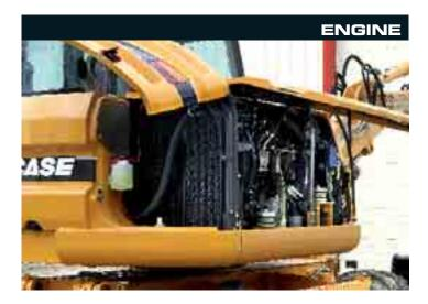
Electronically-controlled turbo charged diesel engine meets Tier III emissions regulations. In tests the 99 hp (74 kW) engine offers increased productivity and lower fuel consumption. Engine and hydraulic pump monitoring and control system offers multifunction use with high output, increasing productivity and tonne/litre output for the customer.
