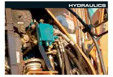
Case has been a manufacturer of class-leading excavators for many years and the WX95 Series 2 builds on that success. The hydraulic system has on-board computer and engine speed sensor control to maximise hydraulic flow and pressure to meet the operator's needs. A swing pressure control offers the driver outstanding controllability, while the flow pump saving circuit minimises oil return to ensure smooth flowing movement of the boom and dipper arm.
