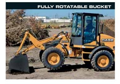
The Case quick coupler, which is standard on all compact E Series wheel loaders, allows for buckets to be completely rotated so that the top of the bucket runs parallel with the ground. This flexibility allows the operator to use the bucket to "pry" the machine out when caught up in difficult, sticky ground conditions. It's also useful for back-dragging material away from foundations, walls or other obstructions.
