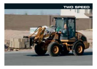
The E Series compact wheel loaders are equipped with an efficient hydrostatic transmission. This provides two speed operation up to 20 km/h on all models. A high speed option on the 121E, 221E and 321E offers a higher speed of 35 km/h.
