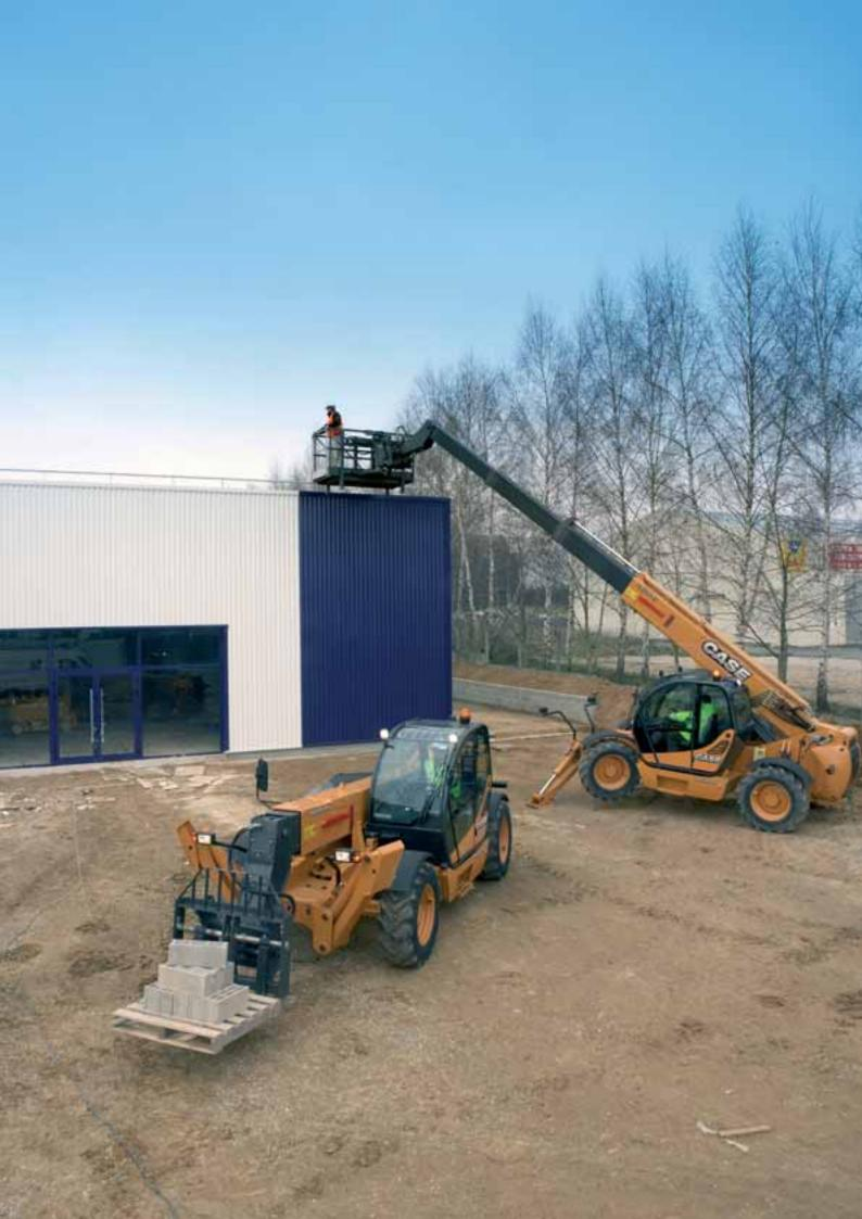
99hp and 188hp (both turbo aftercooled 4,5 liter 4 cylinder Tier 3)
