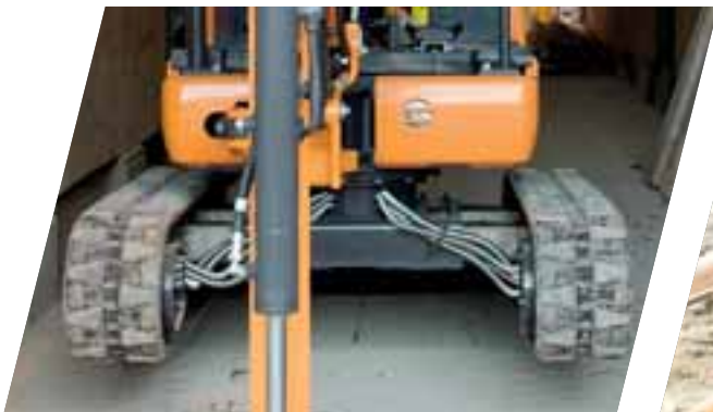
Extended tracks to increase stability while working
