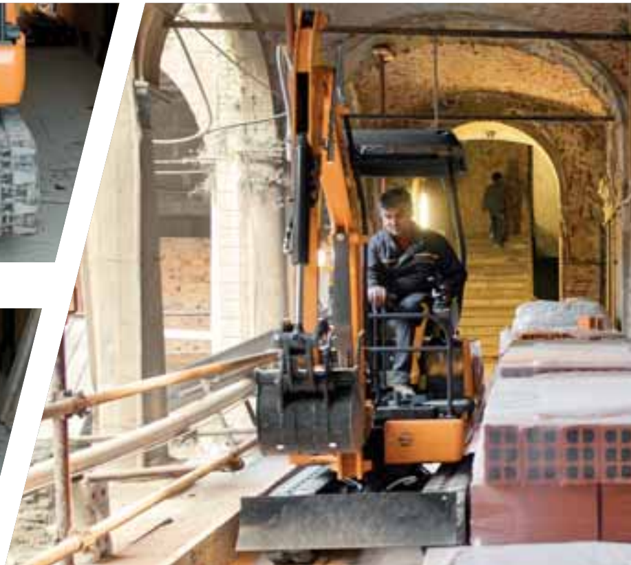
Retracted tracks to access confined spaces
