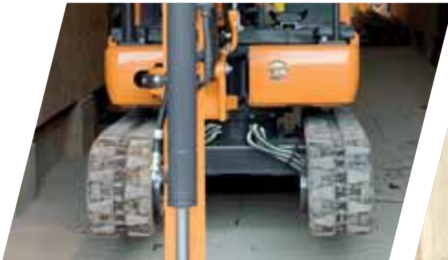
Retracted tracks to access confined spaces
