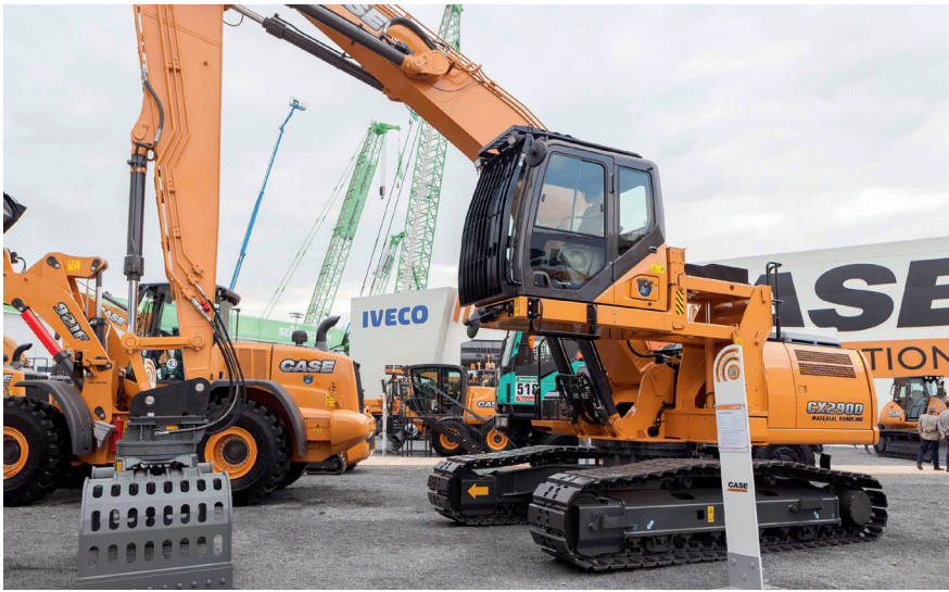
The Case CX290D MH stand 12.5m tall, with a horizontal reach of 11.6m and a lifting capacity of 6.1 tonnes.
