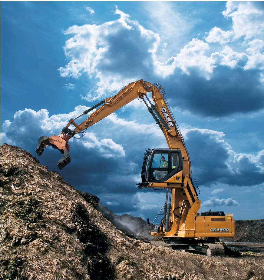
■ The Case CX290D MH with its 5m-high elevating cabin structure, which improve visibility for the operator.
