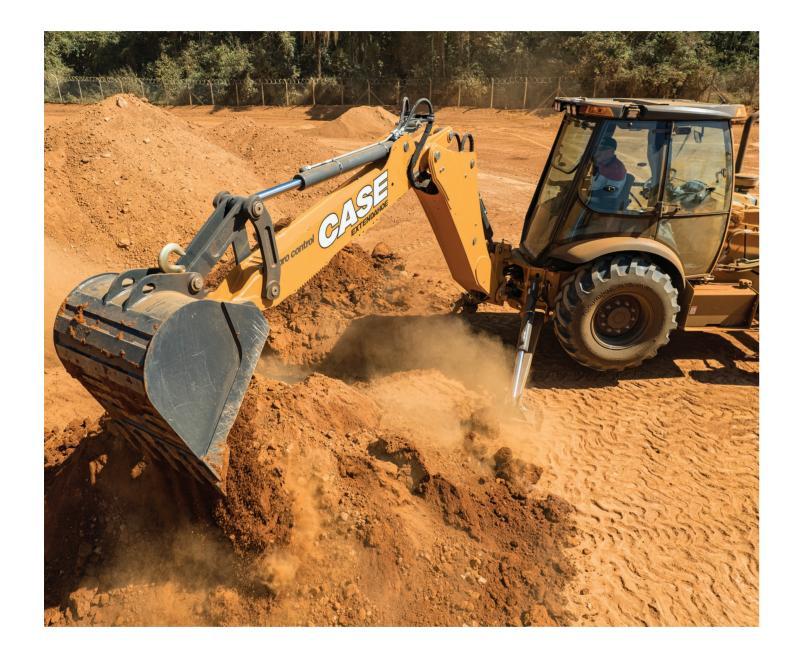
The **580N Series 2 HD** and the **580N Series 2** are equipped with a new hydraulic pump, providing increased speed in operations and command responses. The hydraulic pump offers high reliability and ample power for the most demanding and frequent operations. The hoses and pipes run inside the boom structure, providing enhanced protection.
