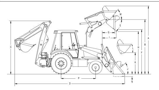
4x4 Traction with 19.5x24 rear tires and 93" general purpose front bucket. \*Standard 4x4 front axle with 12x16.5 tires. \*\*Standard 4x4 front axle HD with 12.5/80x18 tires.
