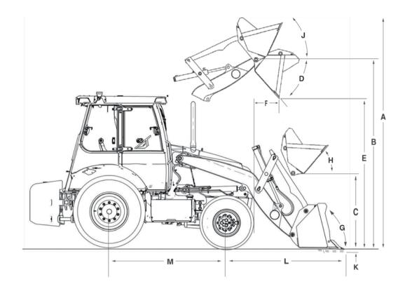
4x4 Traction with 19.5x24 rear tires and 93" general purpose front bucket. \*4x4 Standard front axle with 12x16.5 tires. \*\*4x4 HD front axle with 12.5/80x18 tires.
