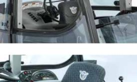
Apart from seats with mechanical suspension, new seats with pneumatic suspension and electric seat height adjustment are available.
