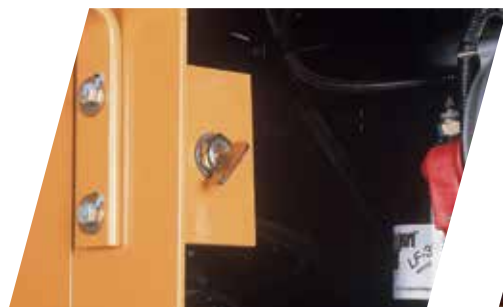
Master switch. This switch guarantee the electrical circuit protection, and is anti-vandalism protection.
