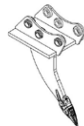
SF5 Tooth (SF5TV): 84318735 Pin (SF5P): 84318739 Adapter (SF8025M5): 84318729
