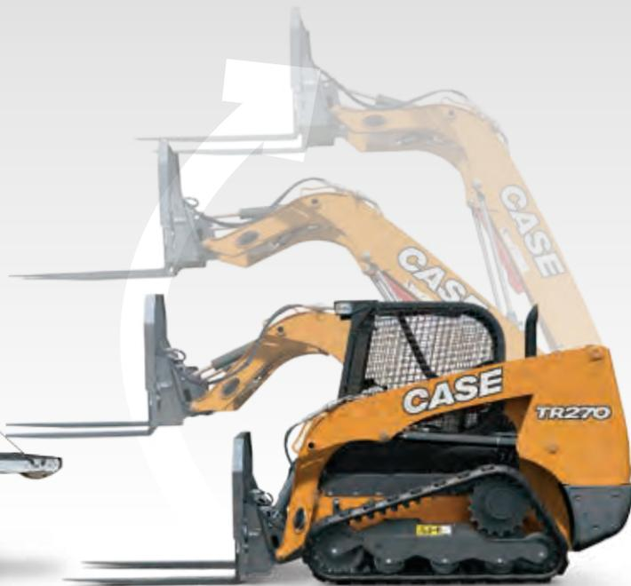
Radial-lift machines are engineered for digging, prying and pushing. The angle of the arm ties directly into the chassis for superior strength when digging and pushing. It also provides maximum reach at the operator's head height, making it perfect for loading and unloading pallets from trucks.
