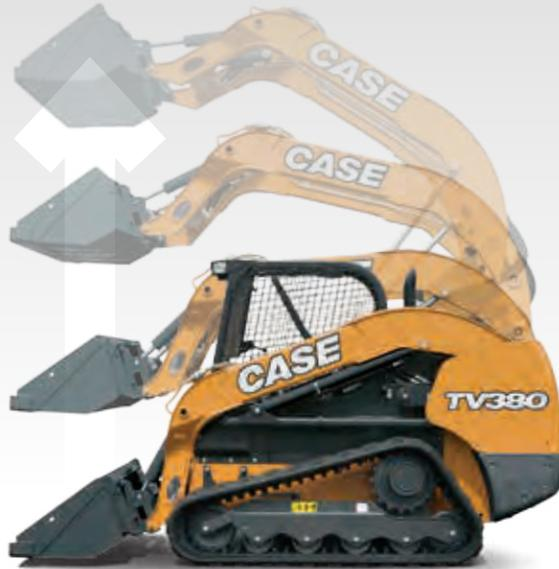
Vertical-lift machines are engineered for lift-and-carry and truck-loading jobs. The geometry of the dual arm allows the load to rise directly up, providing maximum reach at full height. Vertical-lift machines are ideal for reaching over the side of and into the middle of high-side trucks.
