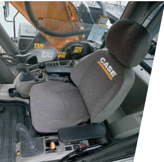
Air suspension seat comes standard.
