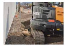
**GET UP IN THERE** The true zero tailswing design allows the operator to work confidently against structures and in tight places — all D-series mini's have zero tail swing with the standard counterweight.
