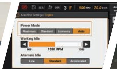
**LOAD-SENSING HYDRAULICS (4 POWER MODES)**
