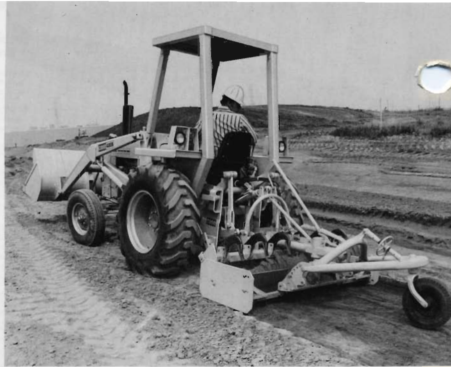
Mod Hitch system for 3-point hitch and rear-mounted equipment.
