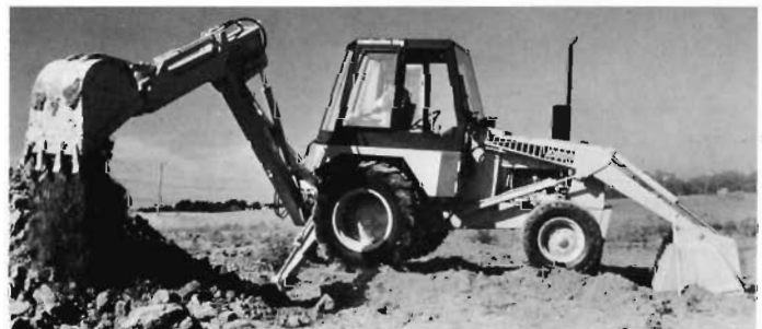
Optional 12'-15' Extindahoe digs deeper, loads high-sided trucks.
