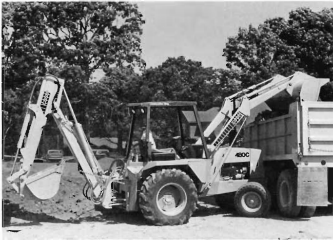
Loader has a 3,000 lb. lift capacity to full height.
