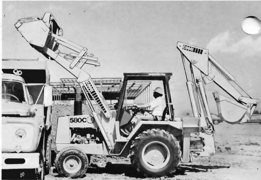
Self-leveling loader keeps payloads moving.
