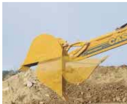
For extended straight wall trenching and improved load retention, Series 2 Super L's now feature 200° bucket rotation.
