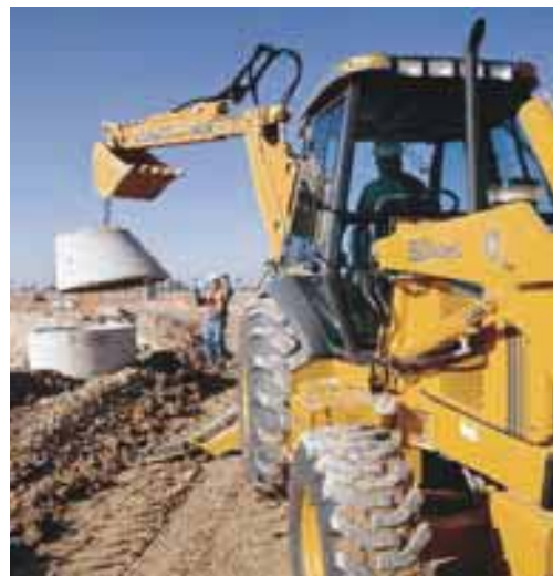
Series 2 Loader/Backhoes have exceptional craning power even with the Extendahoe® dipperstick extended.
