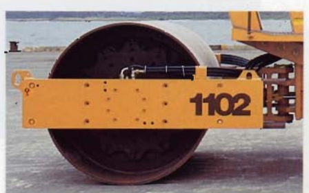
Vibrator and ground drivemotors are recessed into drum for working close to graded areas, curbs or sidewalks.
