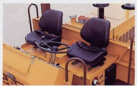
Adjustable steering control can be moved on slide rail to either side of compartment for excellent drum edge visibility.
