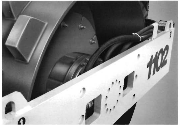
Vibrator and ground drive motors are recessed into drum.
