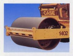
Good Side-wall Clearance Vibrator and ground drivemotors are recessed into drum for working close to graded areas, curbs or sidewalks.
