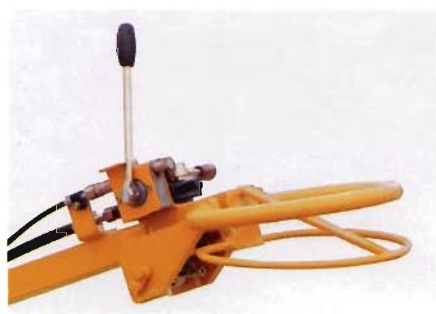
Eccentric vibrator is engaged by mechanical clutch lever.
