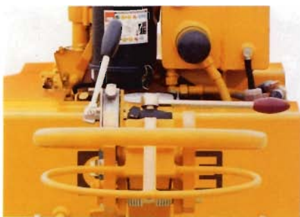
Automatic control stops machine when operator releases steering handle.
