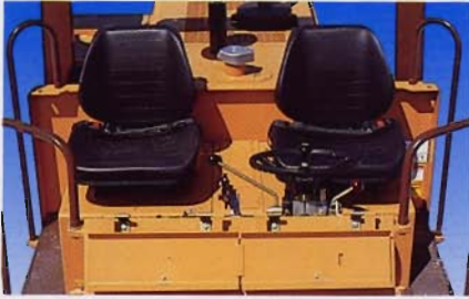
Dual operator seats for optimal operator comfort and visibility.
