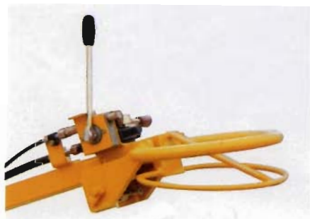
Eccentric vibrator is engaged by mechanical clutch lever at operator's station.
