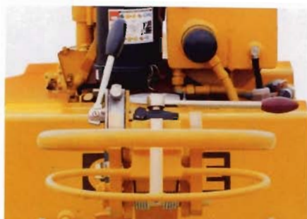
Automatic control stops machine when operator releases steering handle.
