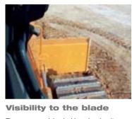
The narrow modular dashboard makes it easy to see the heel of the blade and gauge material flow under the blade.
