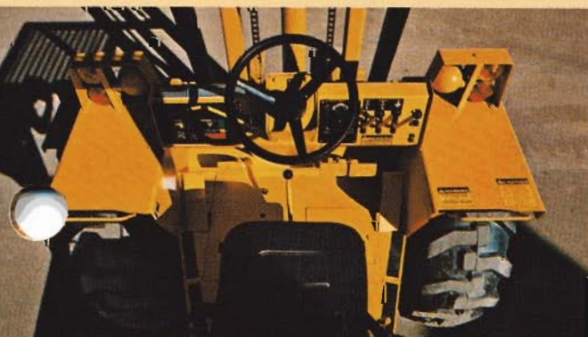
Walk-through compartment is designed for maximum comfort, job visibility and operating convenience. Seat and controls are located high and well forward — providing an ideal vantage point for picking up loads and depositing them on scaffolding or high stacks. Sloped hood and integral counterweight improve visibility to the rear.
