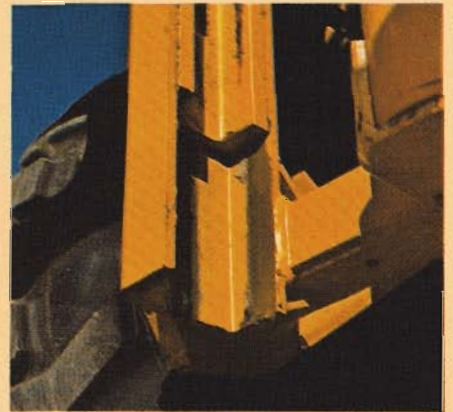
Case forklifts feature slider-type masts with narrow channels for maximum visibility. Bronze wear strips help insure stability at all lift heights. Hook-type carriages provide exact fork placement. Optional side shifter can speed up loading and unloading by shifting 3" (76 mm) either way of center to line loads up without moving the vehicle. Available for all masts except 28' (8.5 m) mast.
