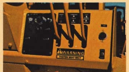
Mast controls, located within easy reach at operator's right, are engineered to minimize effort required for lift, tilt and optional sideshift functions.
