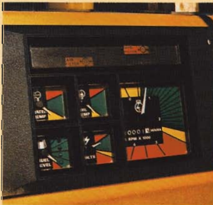
Instruments and gauges have printed circuitry and are clustered in a vandal-resistant plug-in module. Gauges incorporate international symbols and warning lights for monitoring a variety of operational functions.
