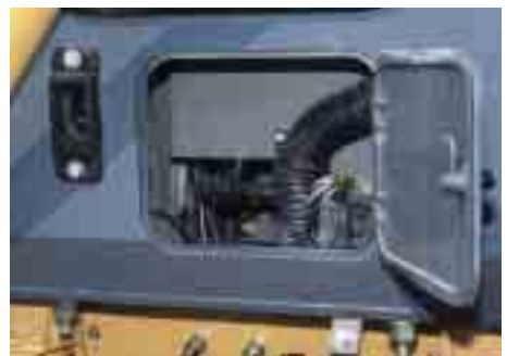
A convenient service door located on the side of the cab allows easy access to electrical connectors without removing interior cab panels.
