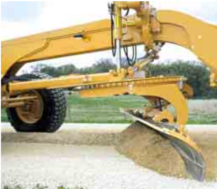
The A-frame drawbar and high-strength circle provide stability, power and maximum turning performance to the moldboard.
