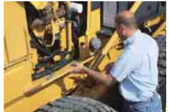
Drop-down side panels improve access to engine components and daily check points.
