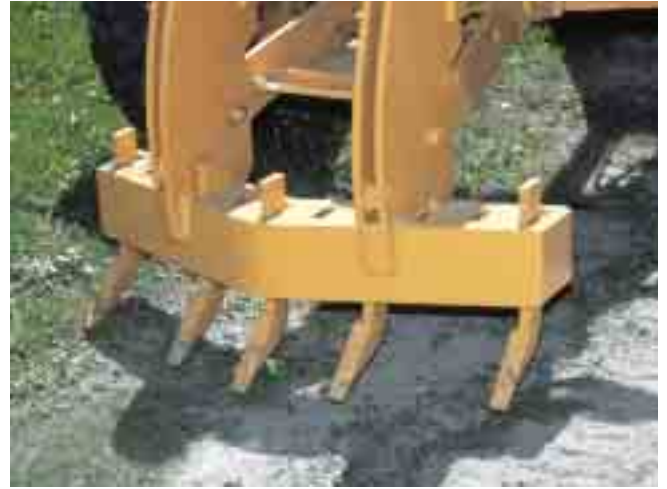
Front scarifier has up to 11 teeth (six standard).
