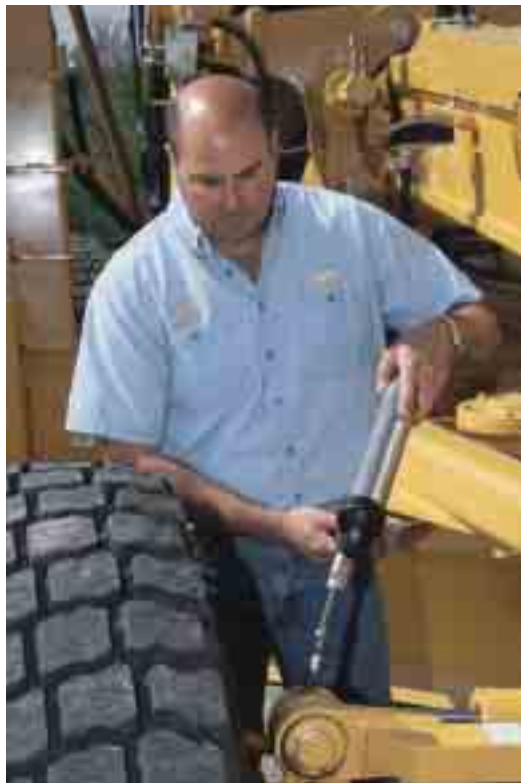
All grease zerts are easily accessed from ground level to speed daily service duties and increase productivity.
