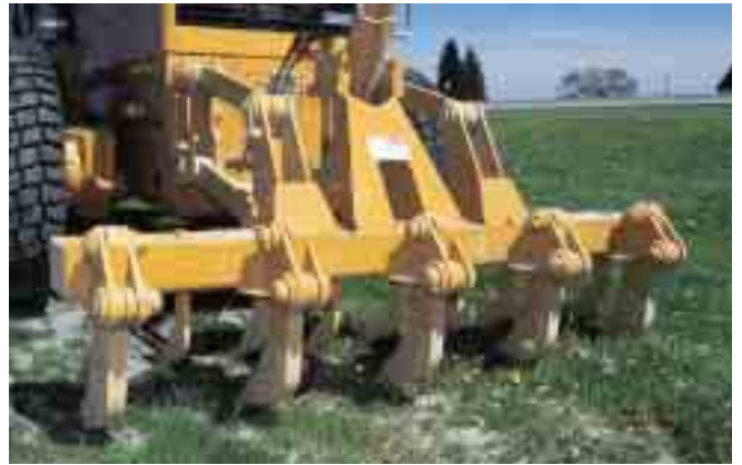
Rear ripper includes up to five teeth (three standard).
