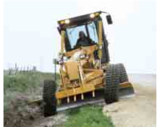
Front wheels lean for traction and moldboard control.
