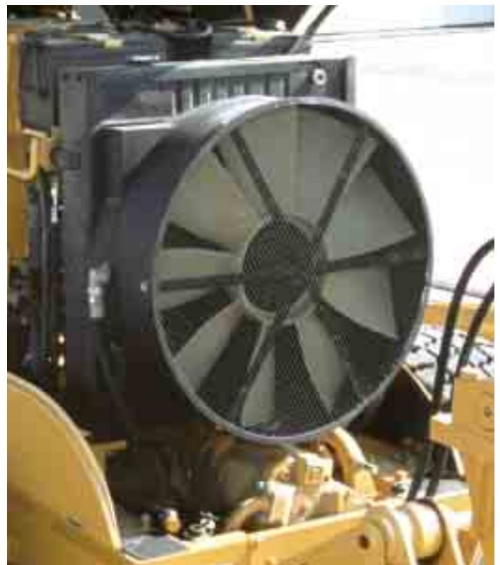
A hydraulically driven fan means a quiet, efficient, cooler-running engine that provides maximum horsepower when tough conditions require the most from your Case motor grader.
