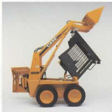
Service ports are located at the rear door, uprights, and under the front floor plate and lift arms, for easy service with no crowding.
