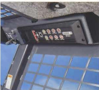
An overhead digital monitor displays vital machine functions, including an hourmeter, fuel level, systems normal light and seat belt reminder.
