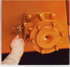
Externally Adjusted Chains and inspection covers allow quick checks of chain tension and simple slidingsprocket adjustments when necessary.
