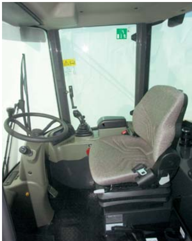
An ergonomic operator environment, featuring tilt column steering and a fully adjustable suspension seat, keeps the operator comfortable through the longest jobs.
