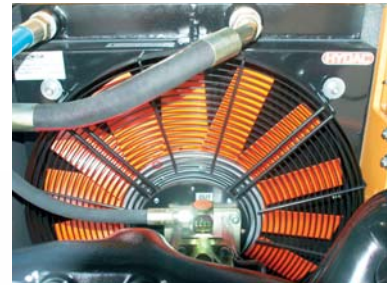
A hydraulically driven fan increases cooling system dependability and reduces noise from the engine compartment.
