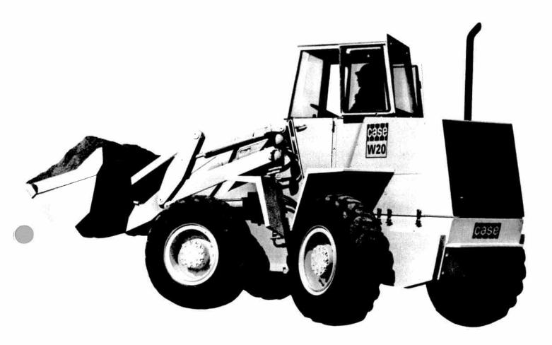
**103 FLYWHEEL HORSEPOWER** Case diesel engine
