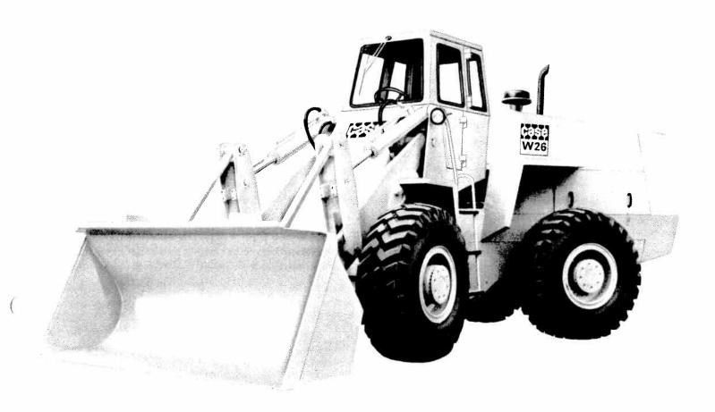
**165 FLYWHEEL HORSEPOWER** Case diesel engine
