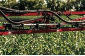
Step 1 Dial to lower pressure selection Perimeter for fewer fines. Spraying . . . . . Interior . . . . **Spraying** 400 kPa . . . . . 4 Bar 15% Fines 25 kph 80 L/Ha 250 kPa 2.5 Bar 5% Fines Step 2 25 kph 80 L/Ha Switch to higher pressure to increase droplet count. . . . . . . . . . . . . . . . .
