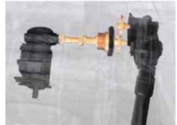
Compact beltless rotor drive with three-speed gearbox for slow speeds in sensitive crops
