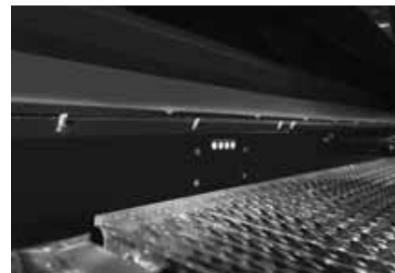
Sieve pressure sensor for high cleaning performance
