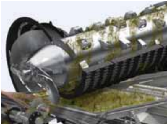
Threshing concaves with 180° wrap angle
