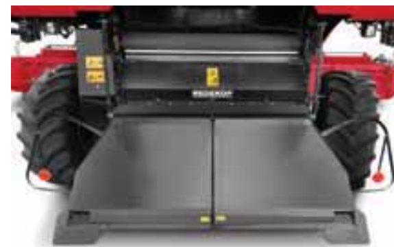
Xtra-Chopping system with independent spreadboards
