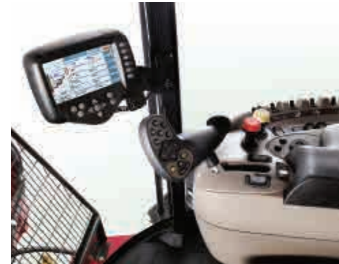
Right-hand side console with multifunction lever
