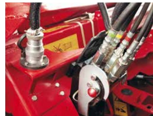
Mount the header in a matter of minutes with the single latch that connects all hydraulic services.
