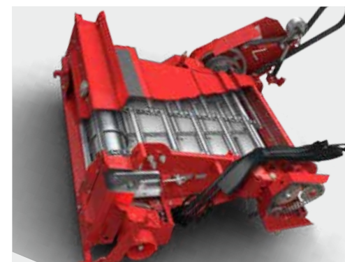
Operate headers up to 9.15m (30ft) with the 80mm lift cylinder option.
