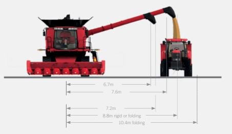
**Standard unloading system** at 113 l/s suited for grain and corn headers up to 12.5m width **High capacity unloading system** at 141 l/s for 7240 and 8240 or 159 l/s for 9240 combines for grain and corn headers up to 12.5m width
