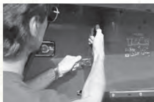
Adjustment for the middle of the chaffer sieve
