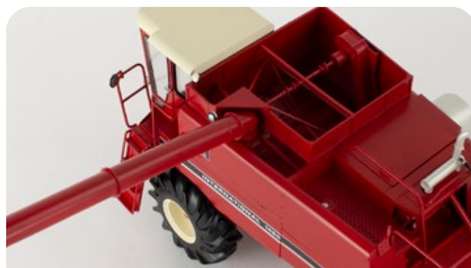
Die-cast grain bin and pivoting unloading auger
