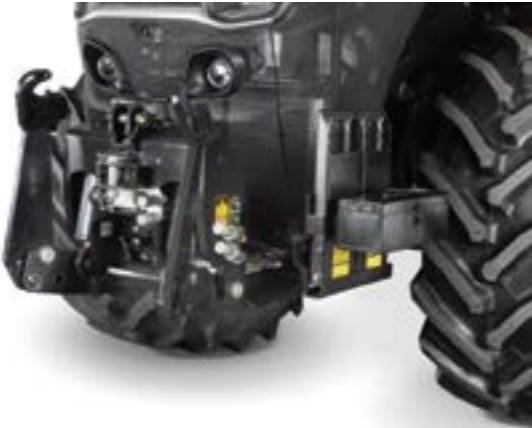
Large range of uses thanks to optional front PTO (1,000 rpm)
