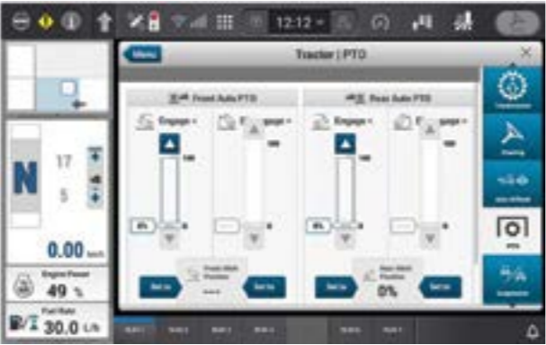
Intuitive layout for the automatic on/off settings for the height-dependant front and rear PTO
