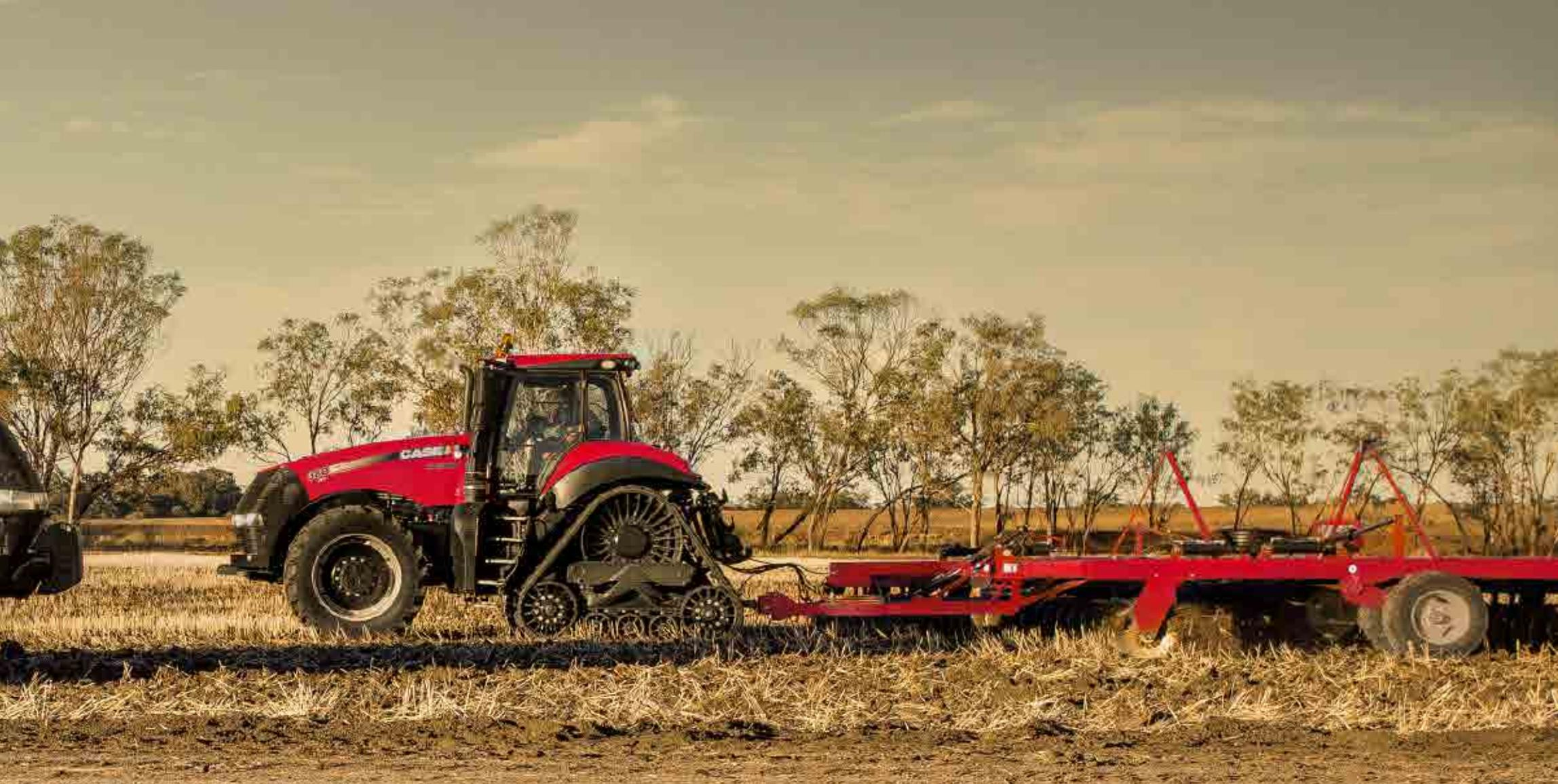
The higher engine power of the new Magnum comes with a PTO to match, as the heavy duty 1,000 rpm PTO delivers its best performance on full engine power. Alternatively, you can opt for the 540/1,000 rpm with interchangeable shafts.
