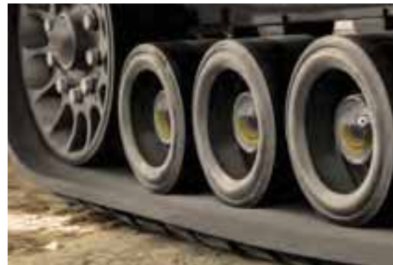
Oil gauge windows in the wheel hubs simplify daily inspections.
