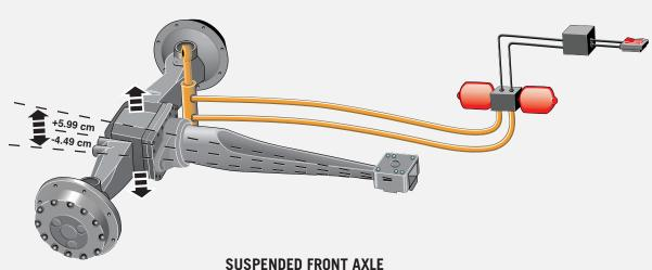
Suspended front axle option provides a more comfortable ride, increased traction and enhanced fuel efficiency.
