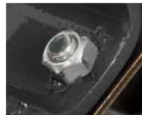
THEIRS: Uneven painted slats which impact torque.
