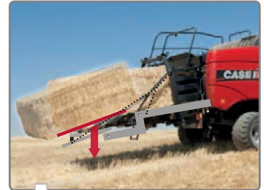
• **Bale weighing kit** accurately measuring the bale weight. The bale weight is recorded and the operator has access to baler capacity and yields.
