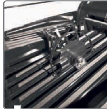
• **The moisture sensor** measures the internal moisture of the bale by utilizing a specialized set of bale length wheels.
