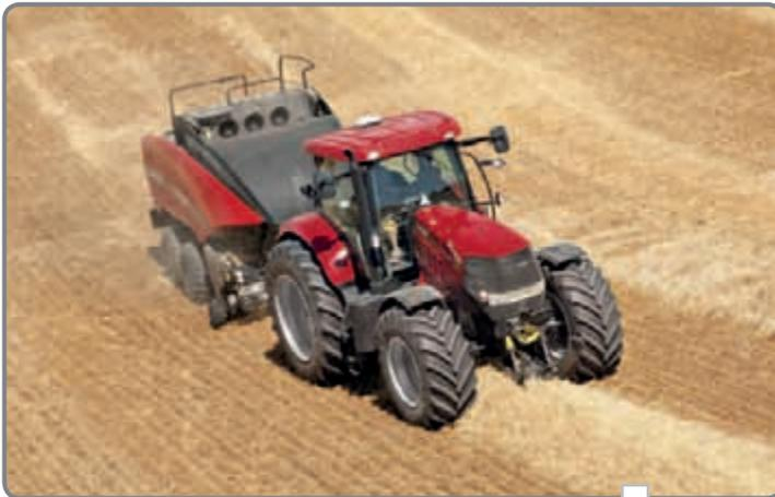
To supply up to date and accurate information to run the baling operation efficiently, **Case IH balers equipped with data collection systems supply detailed and summarized data on the parameters on each bale** (moisture, weight and location on field).
