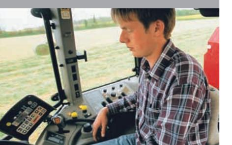
**The ultimate in flexibility.** With the RB electronic system, operators can choose twine or net and change the rolls within a few minutes.
