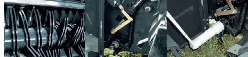
Heavy duty floor roller provides gentle but firm rotation while supporting the weight of the bale.
