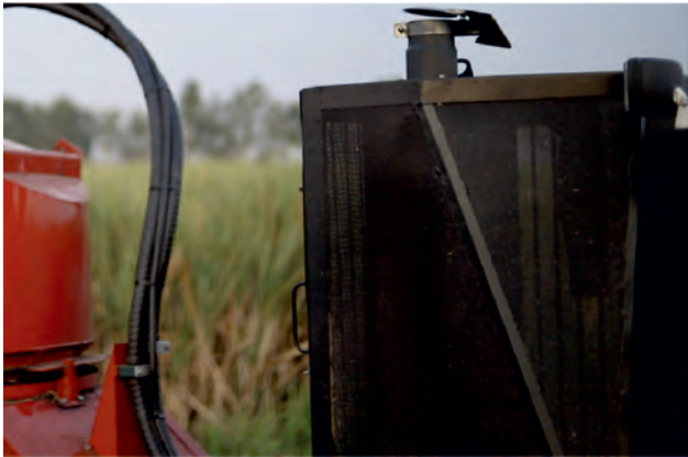
Improved Bird Cage Sealing Engine safeguarded from trash entry, improved productivity & safety
