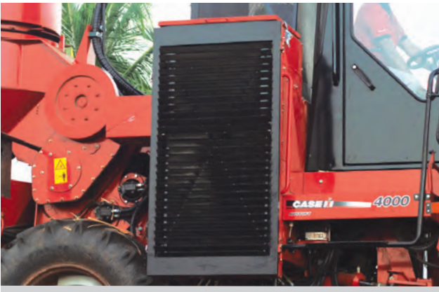
Bigger Radiator Increased cooling efficiency
