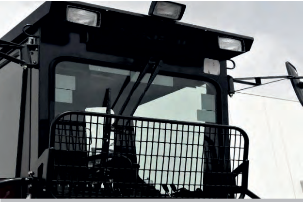
Cabin Windshield Guard Effective protection of cabin windshield from cane hits
