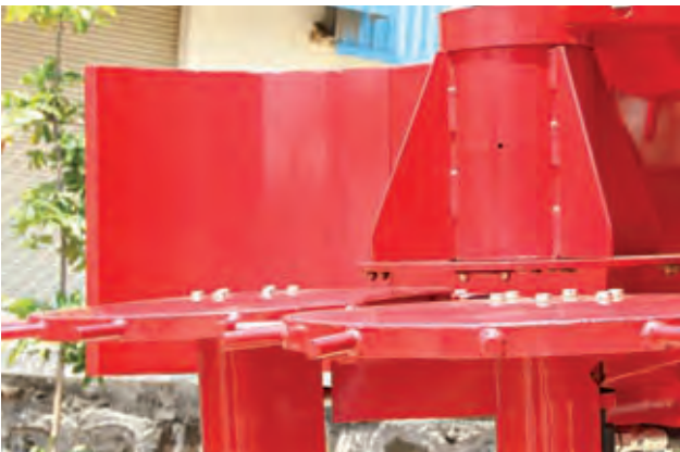
Disc-O-Gather Topper* Ensures excellent removal of Tops resulting in less trash going into machine & reduced fuel consumption
