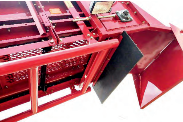
Elevator Rubber Flap Avoids the billets from falling onto the ground during Infielder filling
