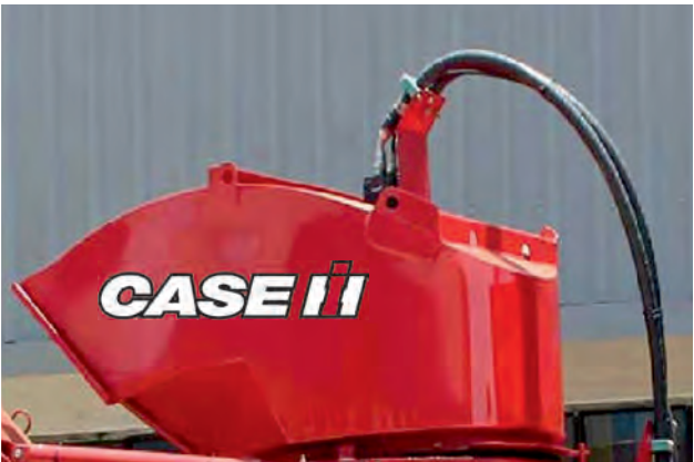
Heavy Duty Extractor Hood Improved reliability of cane trash extraction system
