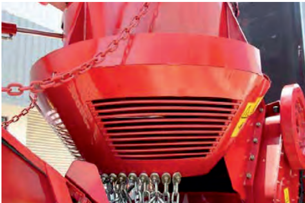
Turbo Air Drag Cleaning System Better extraction of trash resulting in cleaner cane billets
