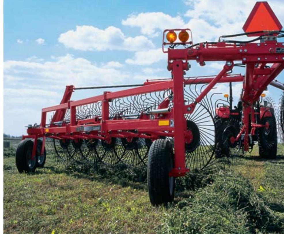
▲ **Articulated steel frames** allows rake to float over uneven terrain.
