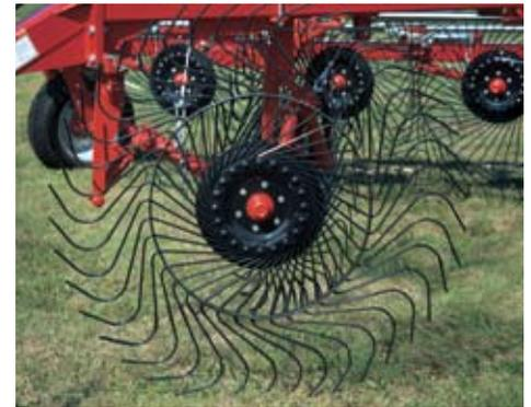
▲ **55-inch diameter raking wheels** each feature 40 equally spaced spring steel finger tines, designed to cleanly rake the most hay and build optimum windrows.
