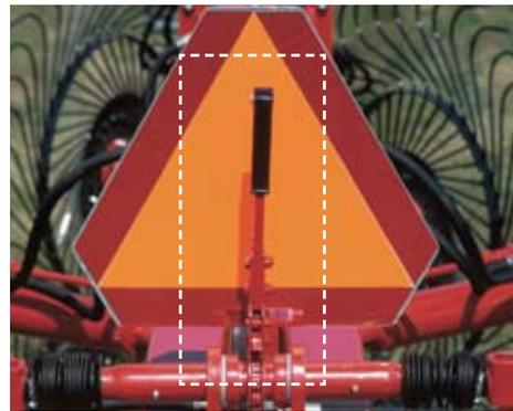
▲ **Easy windrow adjustments:** ratcheting lever adjusts windrow width from 3 feet up to 6 feet on some models. Optional hydraulic kit allows on-the-go windrow adjustment from the tractor.
