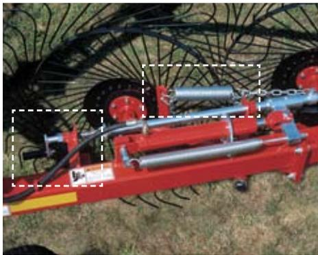
▲ **Quick and easy adjustments:** individual flotation springs on each raking wheel are connected to a central point allowing you to easily adjust the flotation on the entire wheel gang.
