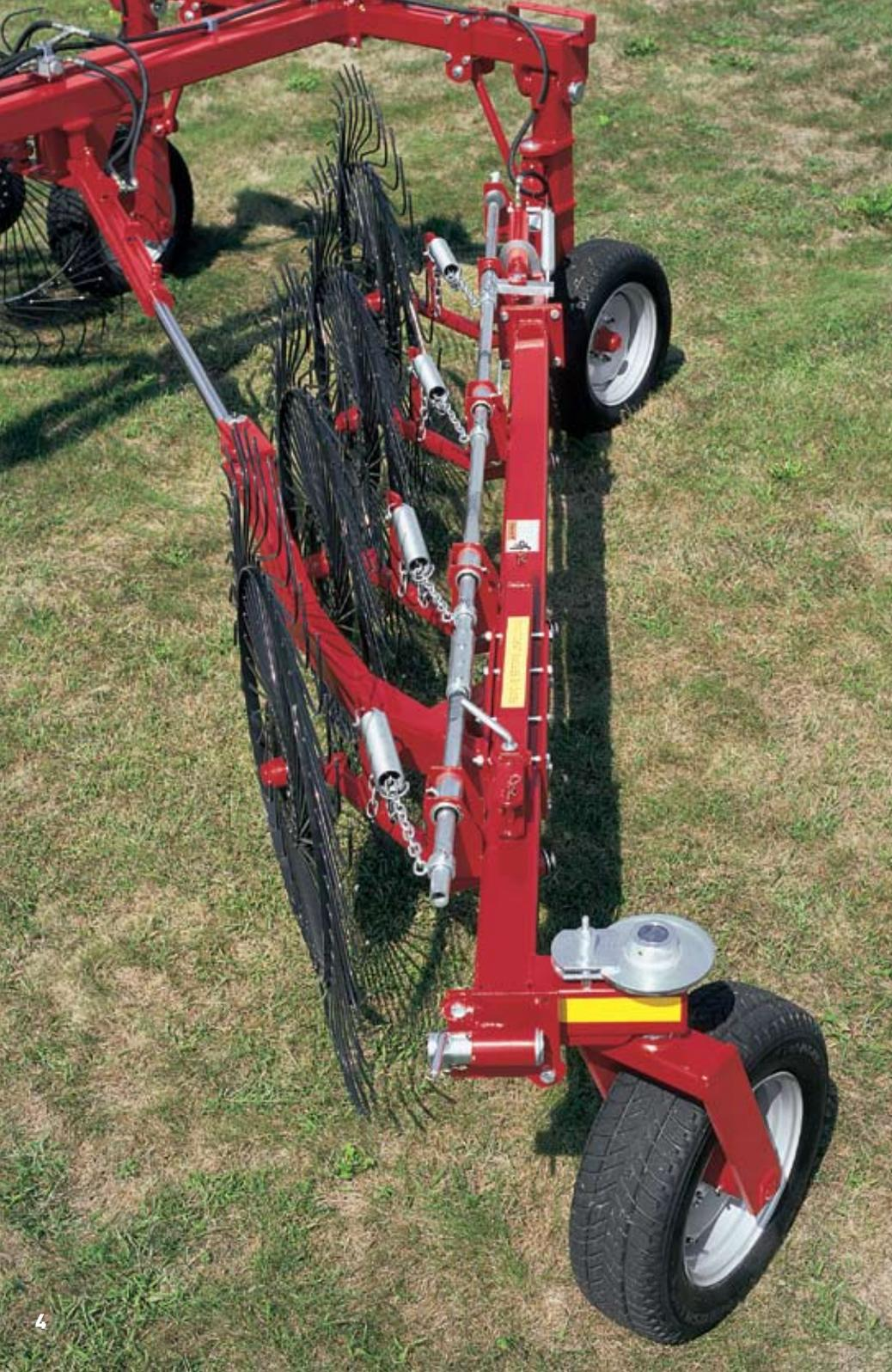
◀ **Swing cylinders** quickly and easily expand raking wheels from transport to working position.
