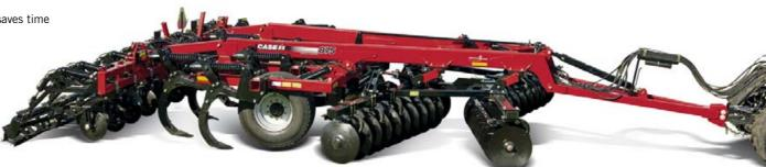
Disk gangs feature spools between the Earth Metal blades, which add weight to increase cutting pressure and clearance for residue flow through the gangs.
