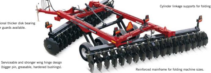
Heavier gang tubes on folding machine sizes.
