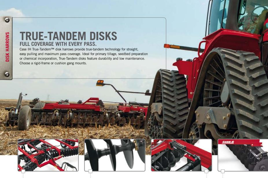
:--- The Pull Frame features an increased section of pull plates and 9.5 mm (375 in.) wall tubing for added durability. • Earth Metal® blades feature a crimpedcenter design for increased blade strength and shallower concavity for better soil penetration with minimized soil compaction. The blades are mounted on nodular cast iron spools for even greater strength and durability. The rockshaft, clamps and angle ....: mounts provide great strength for the weight and size of the True-Tandem 375 disk.
