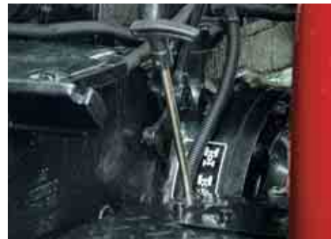
Mechanically actuated, wet disc brakes. Easy to use parking brake – acting on service brakes.
